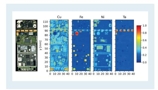
1 Element maps of a mobile phone board measured with LIBS.
