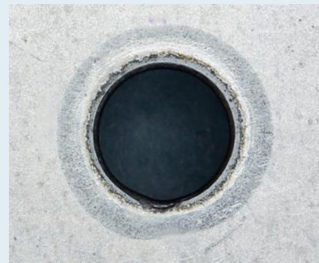
1 Laser edge finishing process. 2 Laser edge finished specimen for hole expansion test.
