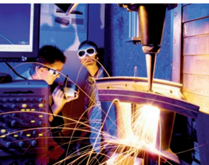
Drilling with Laser Radiation.
