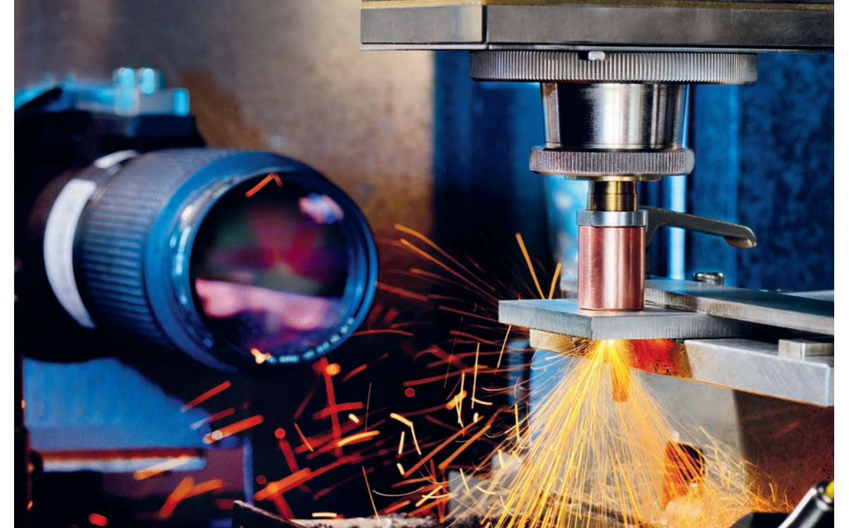
Laser beam fusion cutting with the "cutting whistle".
