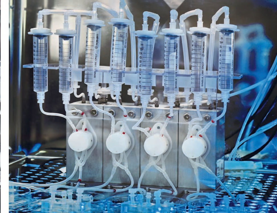
1 OoC of PDMS with intersecting channels separated by a membrane. 2 Cell cultivation in four OoCs with automated perfusion.
