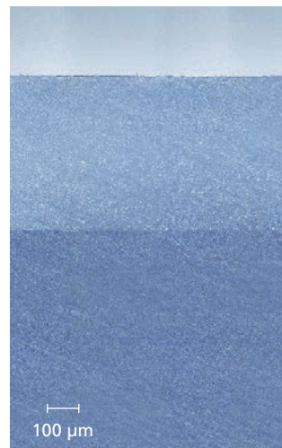
1 Top: Laser-welded PA6.6-GF20 specimen. Bottom: Fracture pattern after tensile shear loading with failure of the base material outside the weld area. 2 Microscopic analysis of the joining plane without any visible damage or heat-affected zone.
