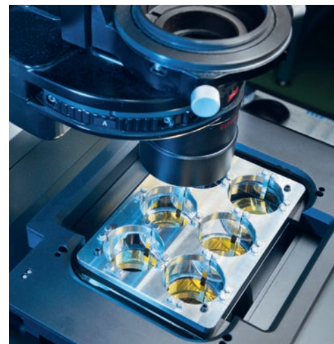
1 Microscope with integrated high-speed image recognition and laser-assisted cell separation. 2 Substrate holder for collecting and cultivating transferred cells in the multiwell cell culture vessel.
