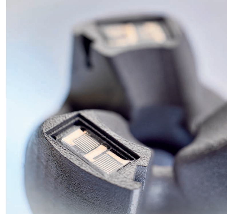
1 Component produced by the LPBF process with integrated sensor technology. 2 Printed strain gauges in incomplete AM component.
