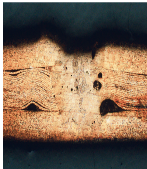
1 Laser-beam microwelding of electrode stacks with a wavelength of 1070 nm.
