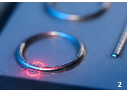
1. Measuring beam (red) for geometry measurement during Laser Material Deposition. 2. Inline measurement of track heights applied by Laser Material Deposition.
