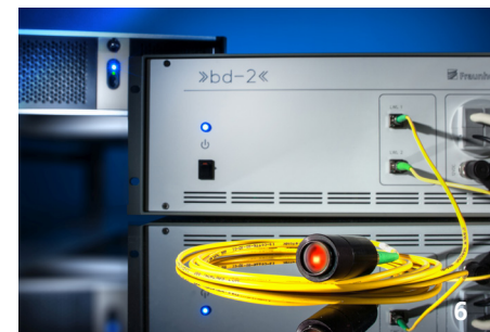
5. C-frame for two-sided distance measurements to determine metal strip thicknesses. 6. »bd-2« sensor technology and data processing electronics with fiber-optical measuring arm.
