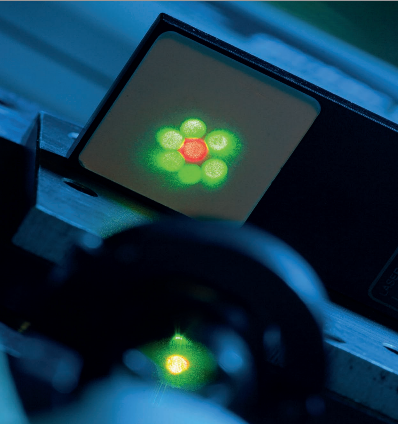
Radiation characteristics of a fiber bundle for laser therapy with optical diagnostics.
