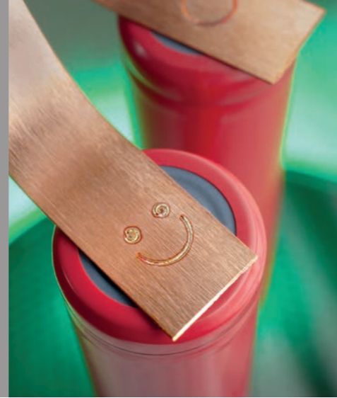
Laser-Based Tape-Automated Bonding (LaserTAB) for welding battery cells.
