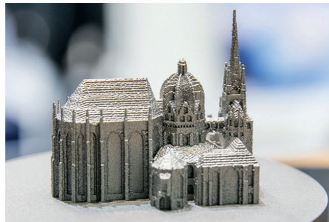
Miniature edition of the Aachen Cathedral, produced with the low-cost SLM system of the »GoetheLab for Additive Manufacturing« of the FH Aachen University of Applied Sciences in cooperation with Fraunhofer ILT.
