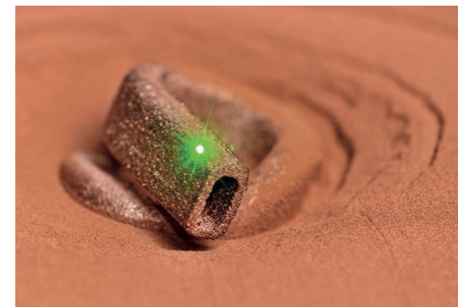
Components made of pure copper: manufactured additively with green light.
