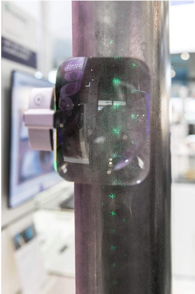
Image 3: Looking through the magnifying glass: Tiny holes drilled with an ultrafast laser in an aircraft wing of the industrial partner Sonaca. © Fraunhofer ILT, Aachen, Germany / Klaus D. Wolf.
