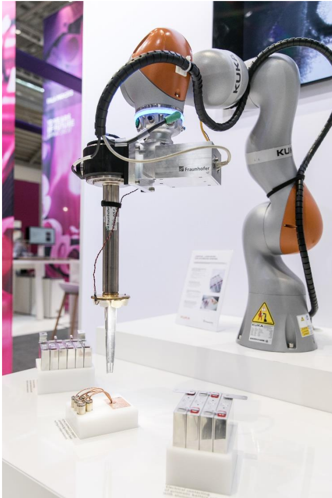
Image 4: In battery technology, lasers already enable precise and stable connections: Laser bonding can be used, for example, to weld copper strips onto battery cells. © Fraunhofer ILT, Aachen, Germany / Klaus D. Wolf.
