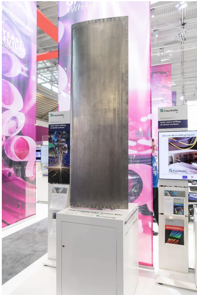
Image 2: The ultrafast laser can be used to drill tiny holes over a large area, for example, in aircraft wings. This reduces air resistance and enables fuel savings of up to 15 percent. © Fraunhofer ILT, Aachen, Germany / Klaus D. Wolf.
