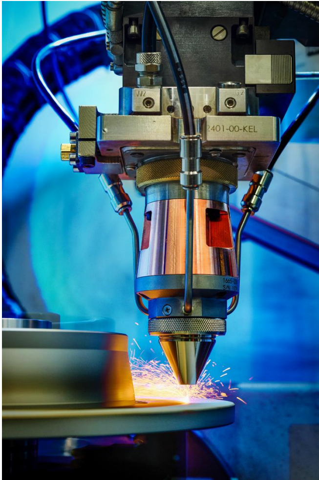
Image 1: Coating a brake disc with the EHLA process. © Fraunhofer ILT, Aachen, Germany / Volker Lannert.
