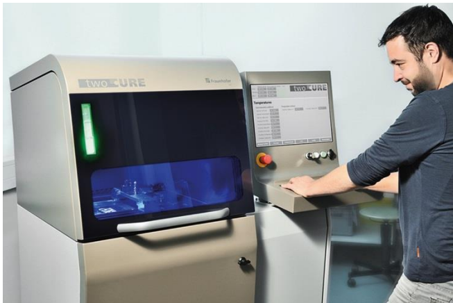
Image 1: At this year's formnext, Fraunhofer ILT will be presenting a "TwoCure" prototype machine for resin-based, support-free 3D printing of plastic components.
