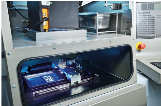
Image 3: Cooled "TwoCure" process chamber with dispensing unit and UV light engine (resolution: 50 \mu\text{m} , 2580x1650 pixel). © Fraunhofer ILT, Aachen, Germany.
