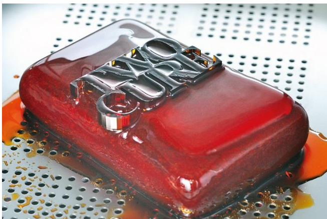
Image 2: By melting at room temperature, the additively manufactured plastic components are released from the frozen blocks.
