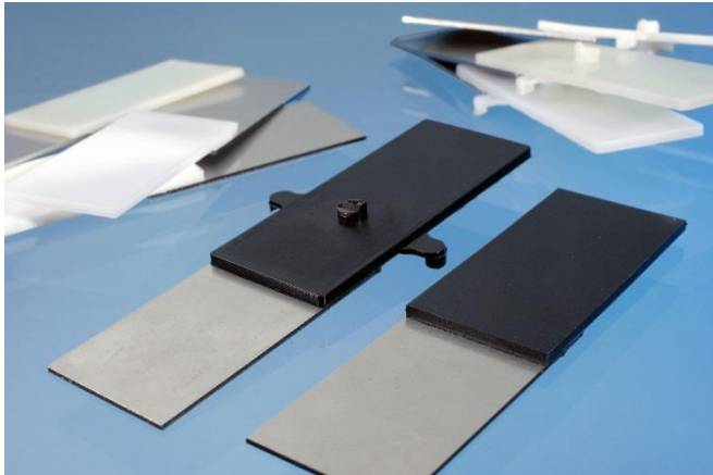
Picture 2: Hybrid bond produced using injection molding. © Fraunhofer ILT, Aachen, Germany.
