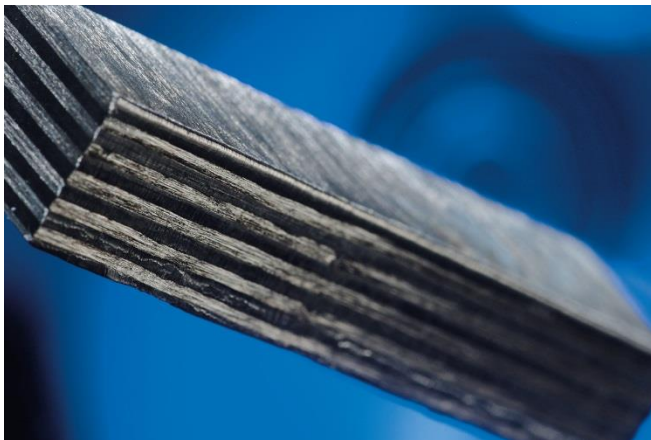
Picture 1: Clean cutting edges in 8 mm thick CFRP pieces are feasible thanks to a high-tech laser process.
