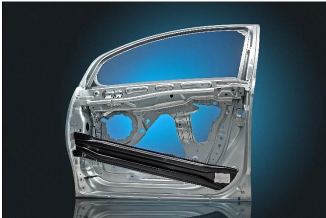
Picture 2: A car door with a FRP reinforcing brace will be on display to demonstrate laser-assisted joining of plastic-metal hybrid compounds.
