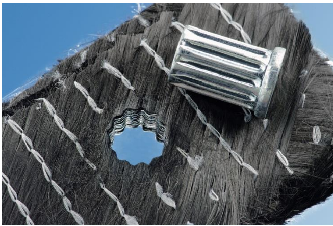
Picture 3: The ultrafast laser drills precise contours into the textile preform, which will later ensure a positive locking connection. © Fraunhofer ILT, Aachen.
