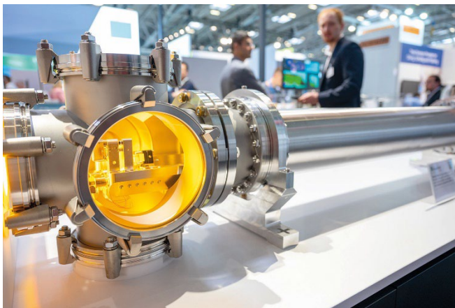
Image 9: The Fraunhofer Cluster of Excellence Advanced Photon Sources - CAPS, high-power USP lasers are developed for industry and research. In the picture: Multipass cell for post-compression at 2 \mu\text{m} wavelength. © Fraunhofer / Markus Jürgens.
