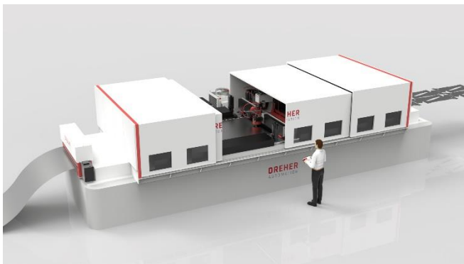
Image 2: Project DIPOOL: The demonstrator of a laser blanking line from Automatic-Systeme Dreher will use new, intelligent AI-supported algorithms to monitor the cutting process, adjust it automatically in the event of deviations and thus ensure cutting quality as well as productivity. © DREHER.
